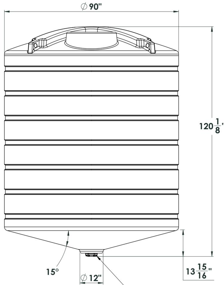
3 inch bolted - bottom drain fitting
