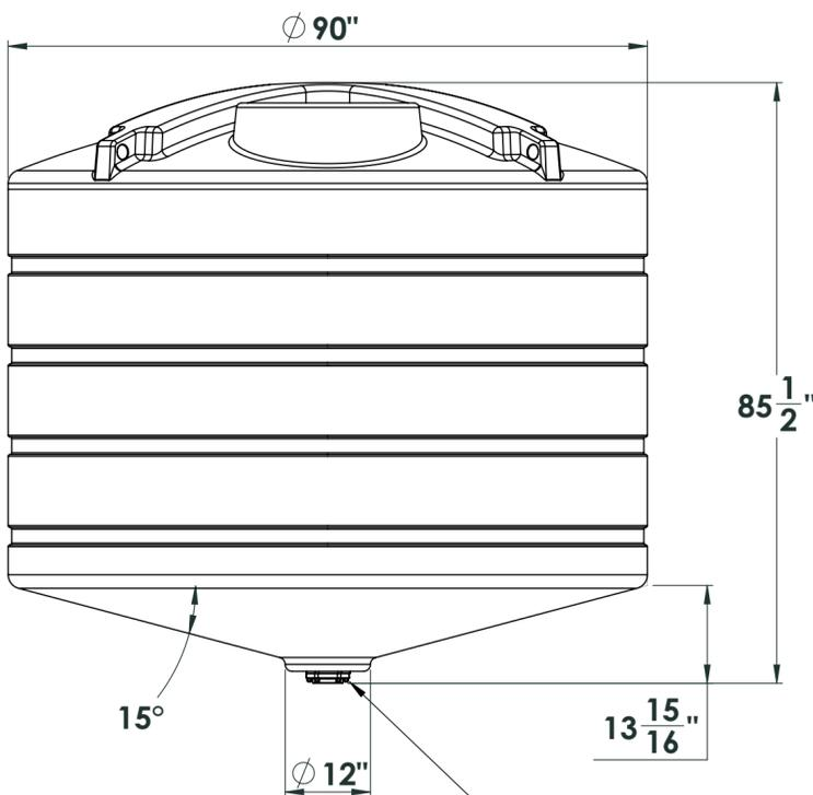
3 inch bolted - bottom drain fitting
