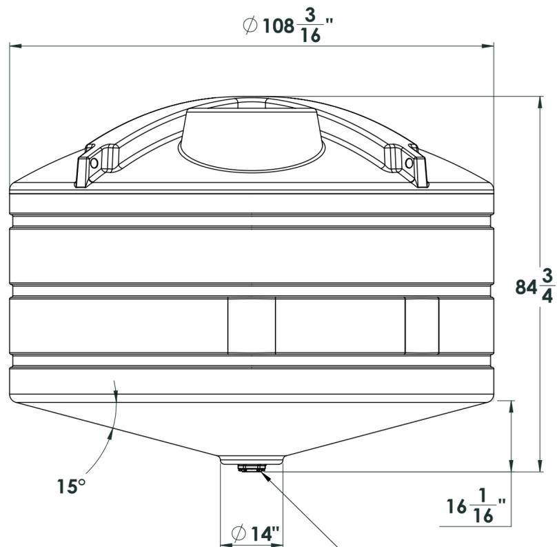
3 inch bolted - bottom drain fitting
