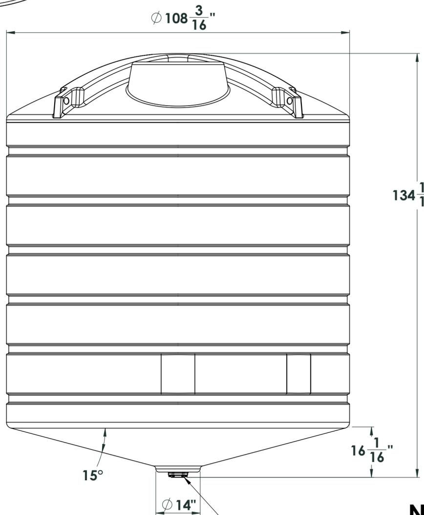
3 inch bolted - bottom drain fitting
