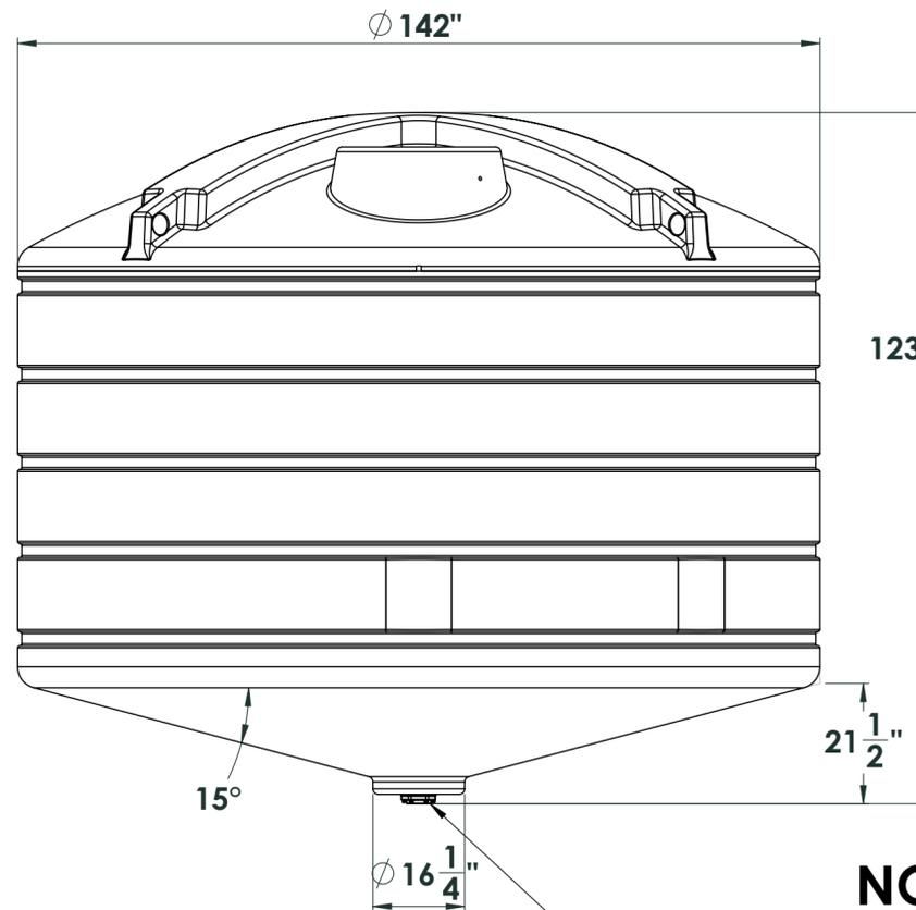
3 inch bolted - bottom drain fitting
