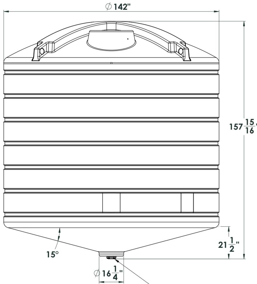
3 inch bolted - bottom drain fitting
