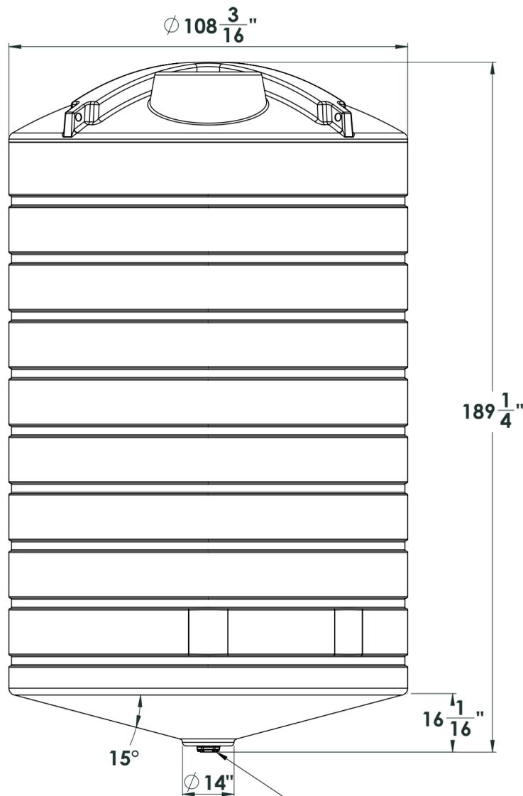
3 inch bolted - bottom drain fitting
