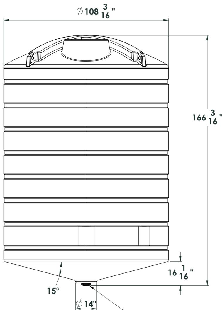
3 inch bolted - bottom drain fitting
