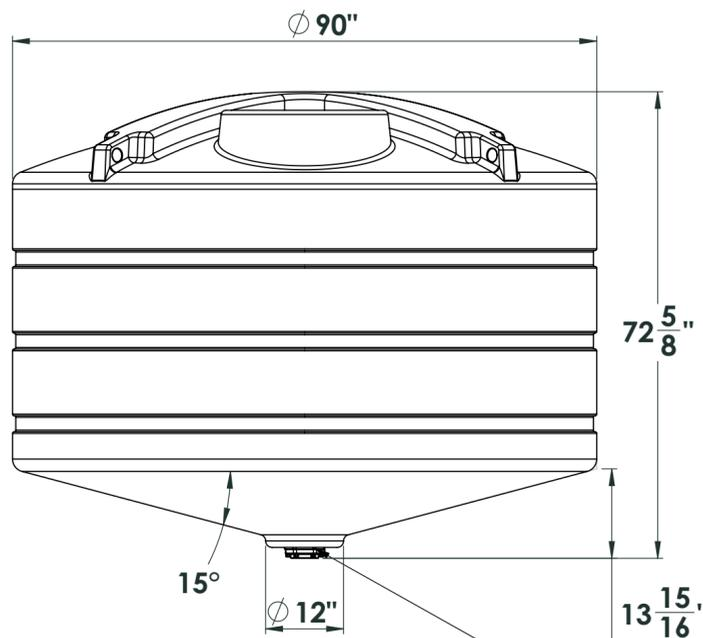
3 inch bolted - bottom drain fitting
