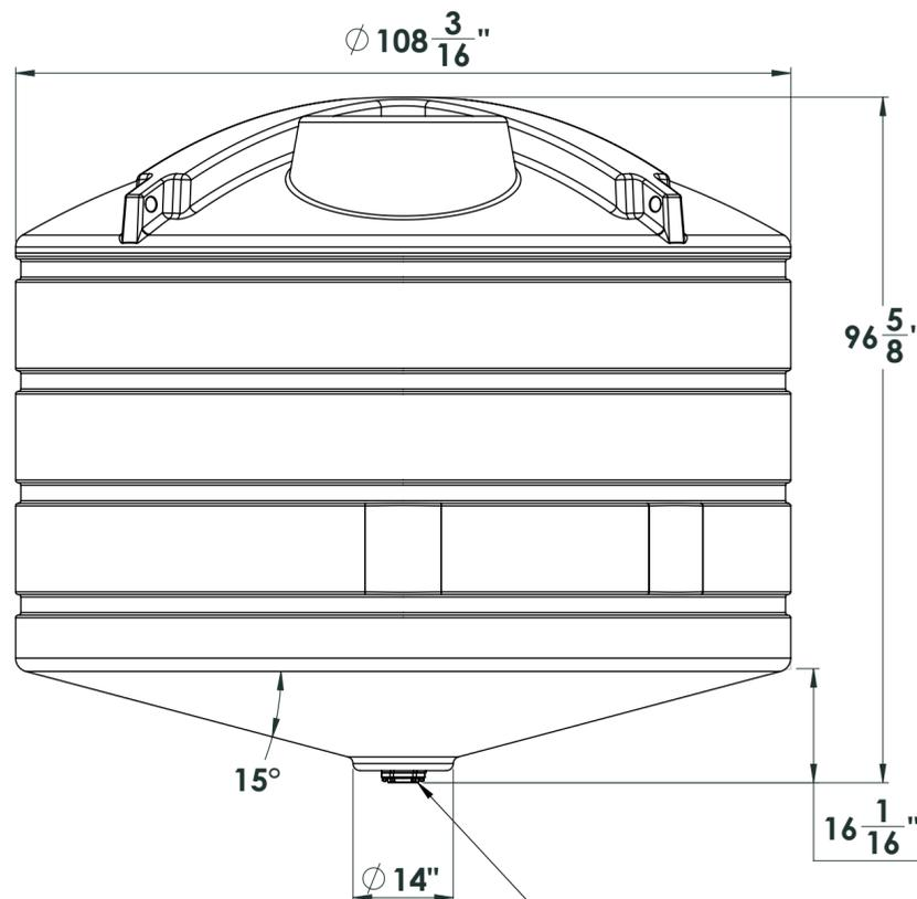
3 inch bolted - bottom drain fitting
