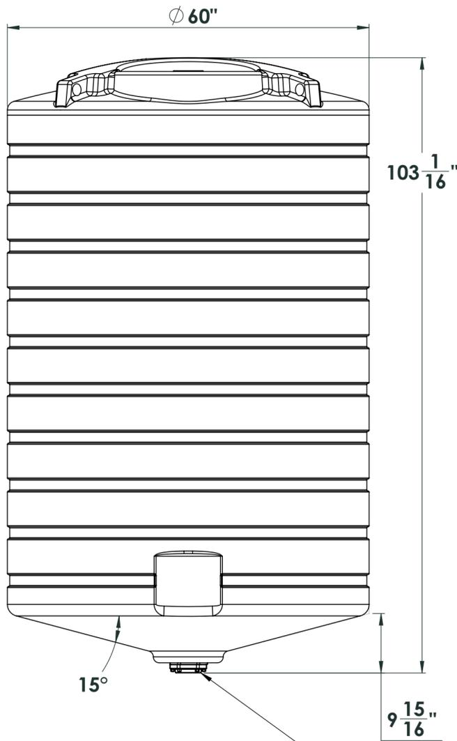
3 inch bolted - bottom drain fitting
