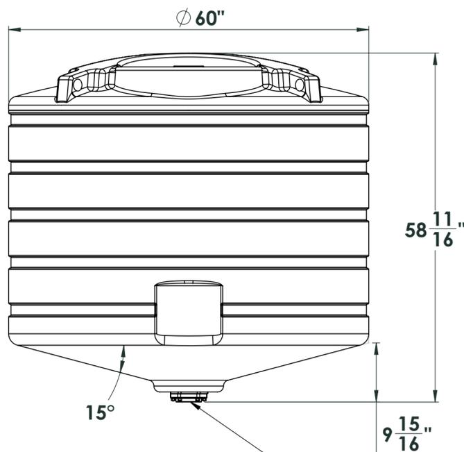
3 inch bolted - bottom drain fitting
