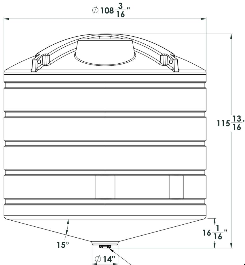
3 inch bolted - bottom drain fitting
