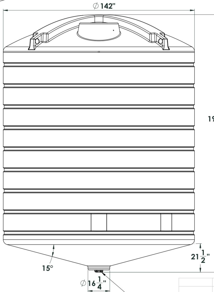
3 inch bolted - bottom drain fitting
